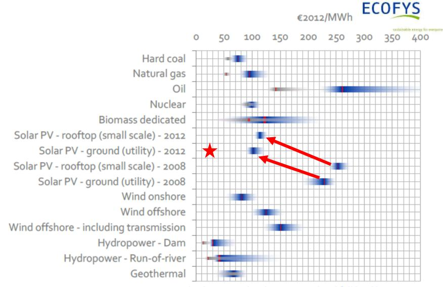
Blue bars: Levelised costs at realised full load hours Grey bars: Levelised costs at technically feasible full load hours
